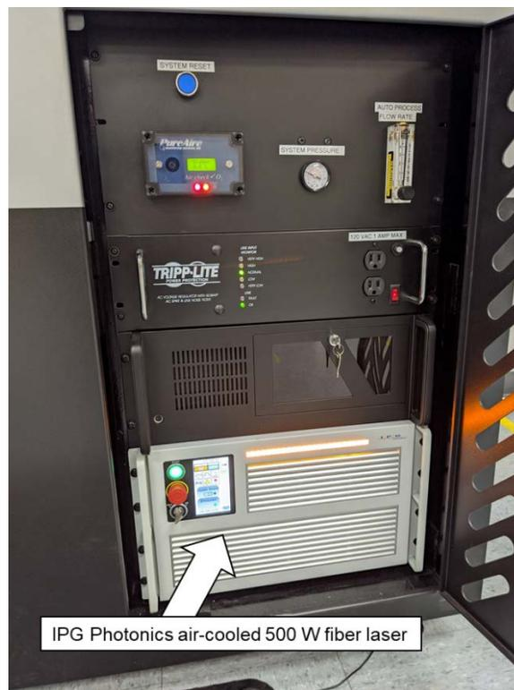
Figure 1. Single laser mounted in PANDA electronics rack
